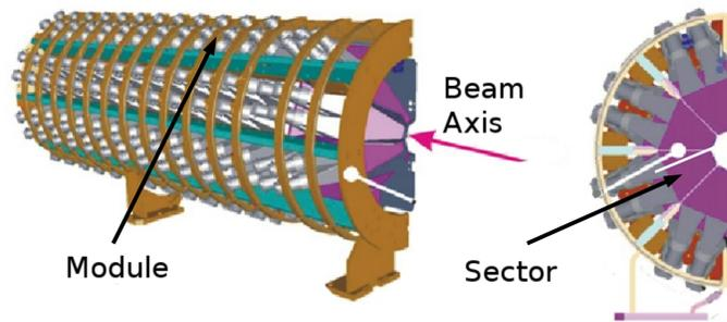
CASTOR consists of two stainless steel skeletons - one for each side of the beam pipe - contain **14 longitudinal sections** (modules), two of them are electromagnetic sections while the remaining 12 are hadronic sections.
